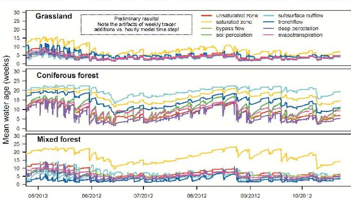
The solute transport routine of HillVi was modified to allow regular virtual time tracer injections into the system via rainfall. Each tracer can be tracked through all storages and fluxes which allows the estimation of time-variant water age distributions and the calculation of mean/median water ages.
