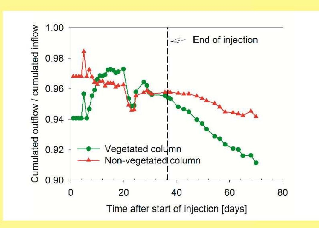
The water balance revealed the intensity of transpiration and hence plant activity and stress following pesticide injection. First, outflow rates of the vegetated column were smaller than in the nonvegetated control due to transpiration losses. After about eight days of continuous pesticide injection, transpiration virtually ceased in the vegetated column, causing larger outflow rates. Apparently, transpiration rates recovered after pesticide and tracer injection was stopped.
