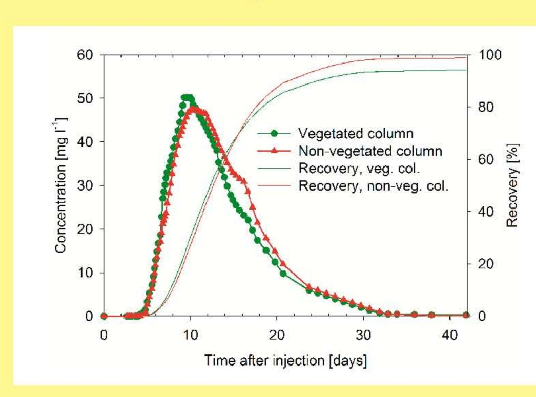
The breakthrough curve (BTC) of the vegetated column peaked higher (50.2 mg l-1) and had a lower (298 h) than the non-vegetated column (47.5 mg l-1, 304 h, respectively). This suggested preferential flow paths along plant roots in the vegetated setup. However, recovery rates were smaller in the vegetated (94.2 %) than in the non-vegetated column (98.8 %). This may be due to plant uptake of bromide, which had already been reported for wetland vegetation (Xu et al., 2004).
