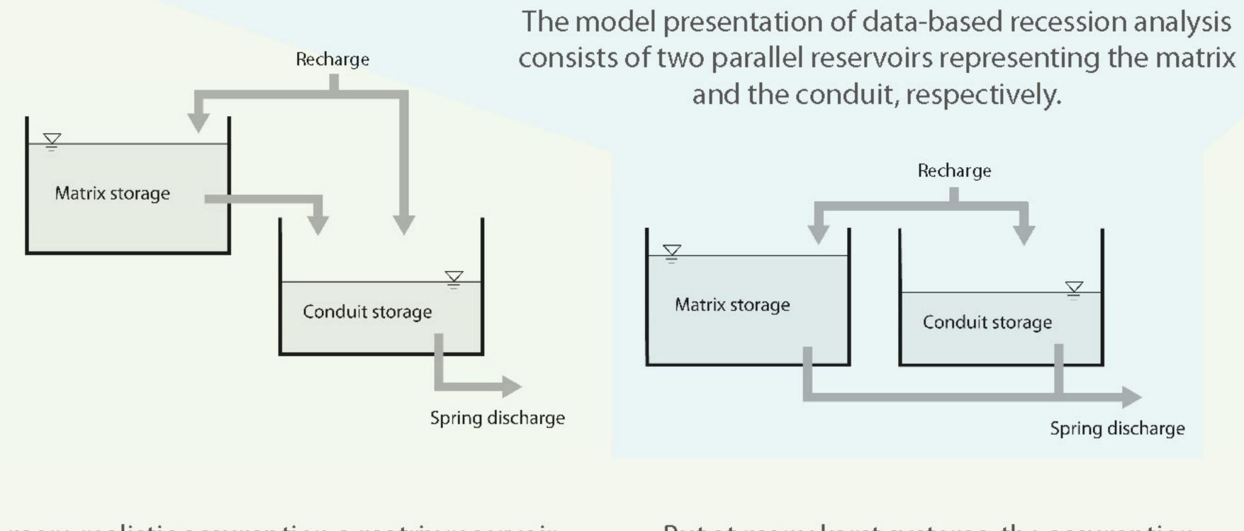
A more realistic assumption a matrix reservoir that drains into the conduits before they discharge at a karst spring.
