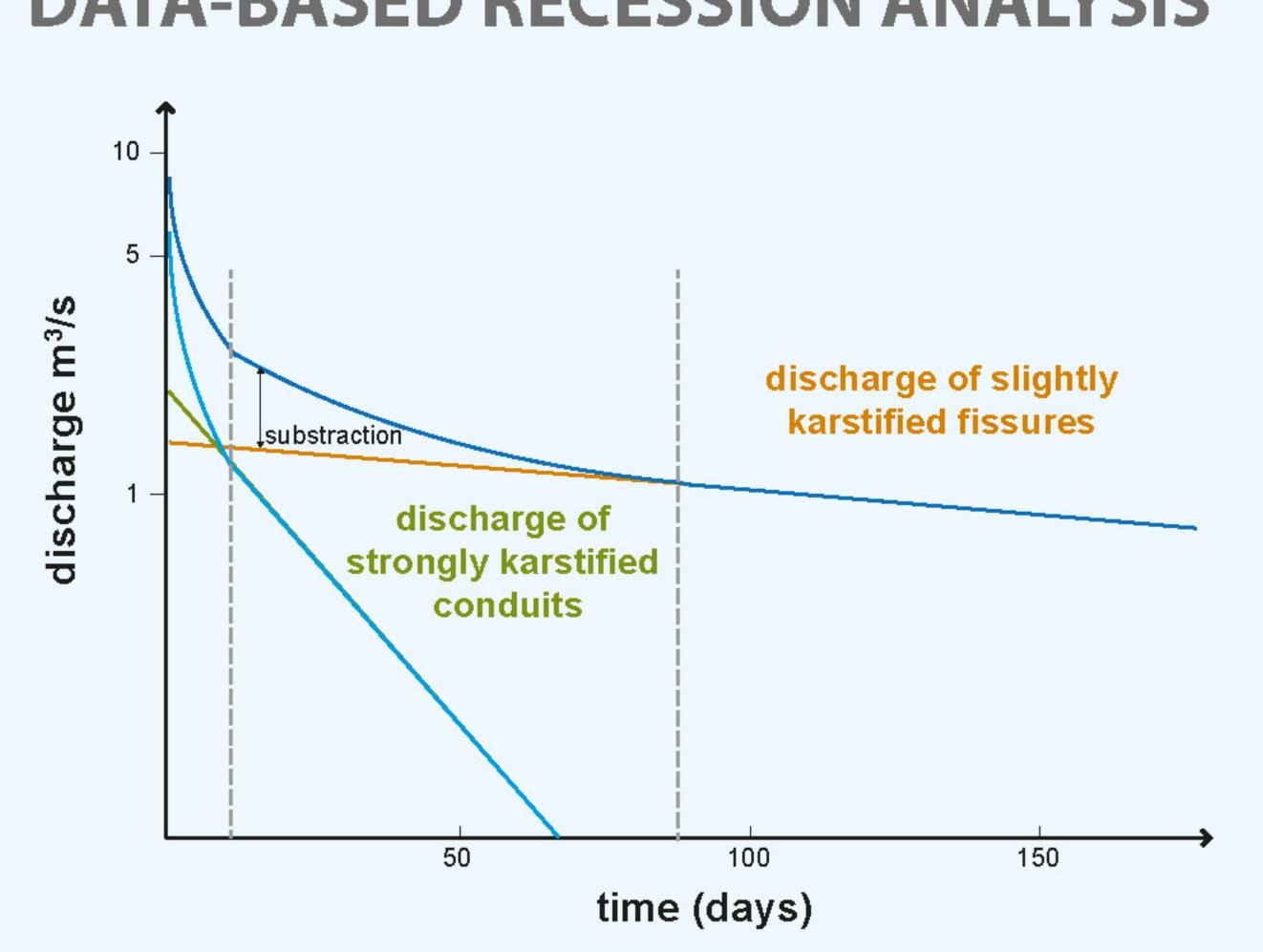
Traditional recession analysis in karst considers the drainage two storages: the fissured matrix and the karst conduits. Plotting the recession limb with a semi-log scale, the part drained by the matrix can be identified by its constant slope. Subtracting the matrix drainage from the recession limb will reveal another constant slope representing the conduits.
