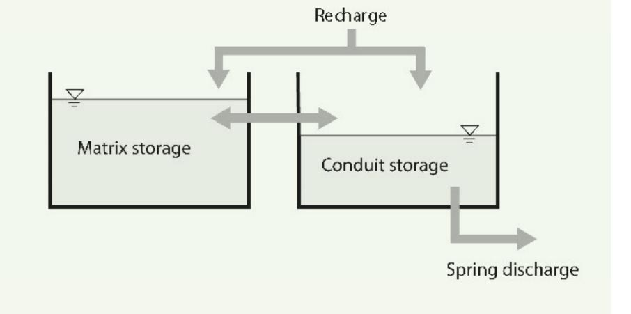
Also, karst systems are known for a dynamic exchange between the matrix system and the conduit system that drains the system.
