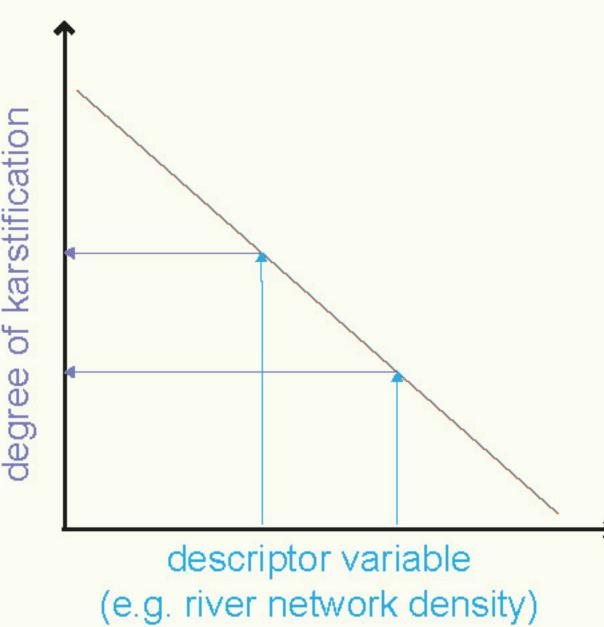
The degree of karstification model-based supported recession analysis will be compared available surface descriptors, e.g. the river network density, to derive large-scale estimates of the degree of karstification over Austria's karst regions.
