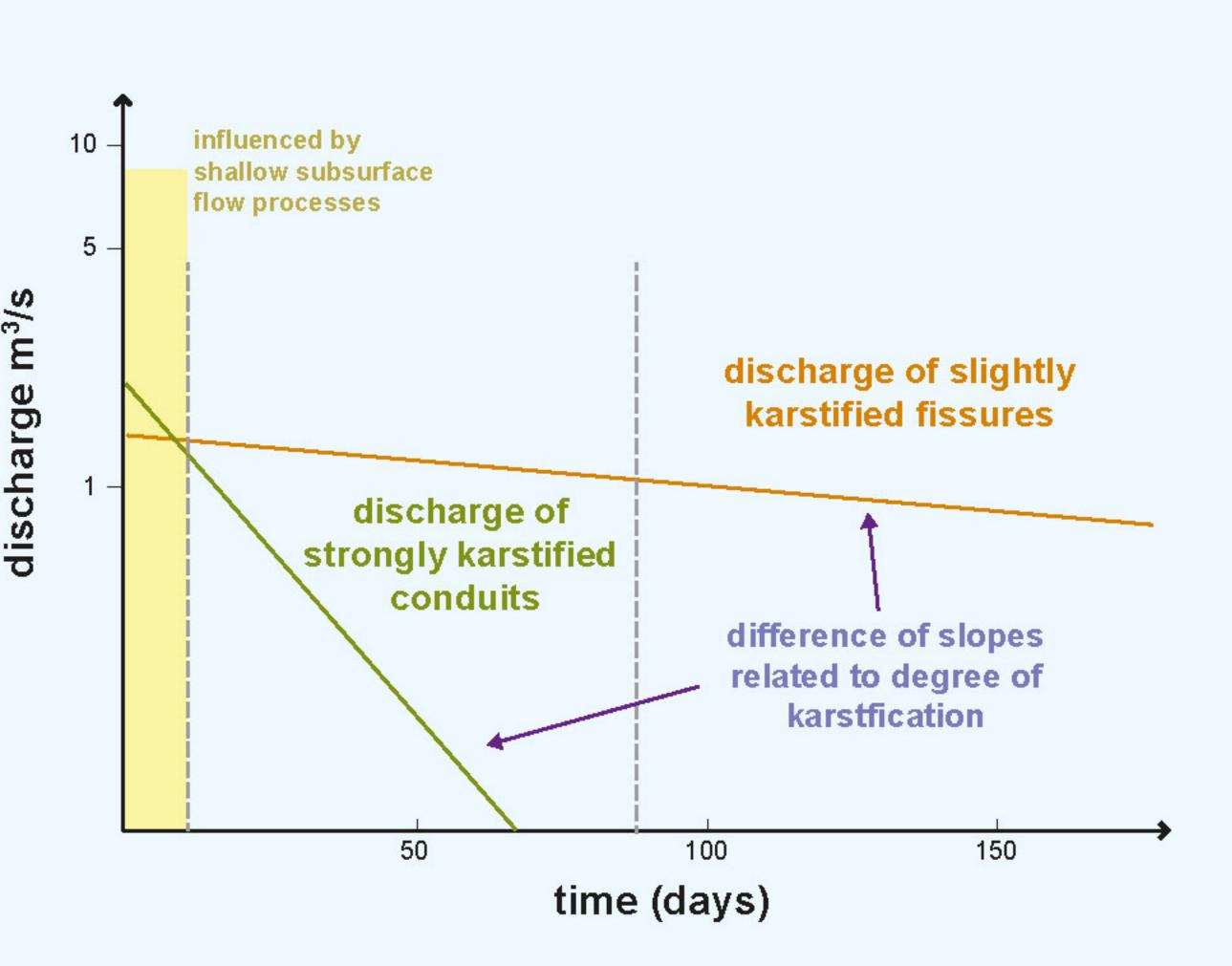
With the slopes of the matrix drainage and the conduit drainage identified, their difference can be used as a metric to quantify the degree of karstifcation.
